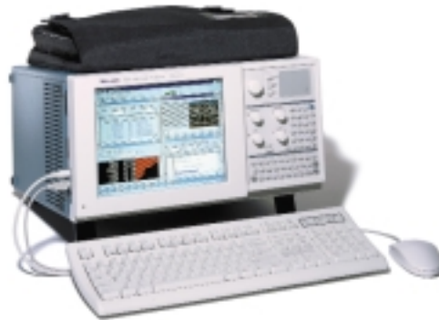
PORTABLE MODULAR MAINFRAME TLA 714 with logic analyzer, pattern generator and digitizing oscilloscope modules
