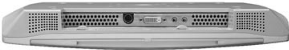
This photo shows the connectors on the bottom of the monitor enclosure.
