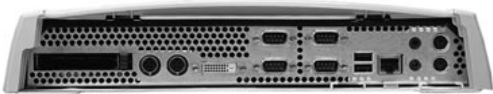
This photo shows location of the connectors and ports in the computer connector bay.
