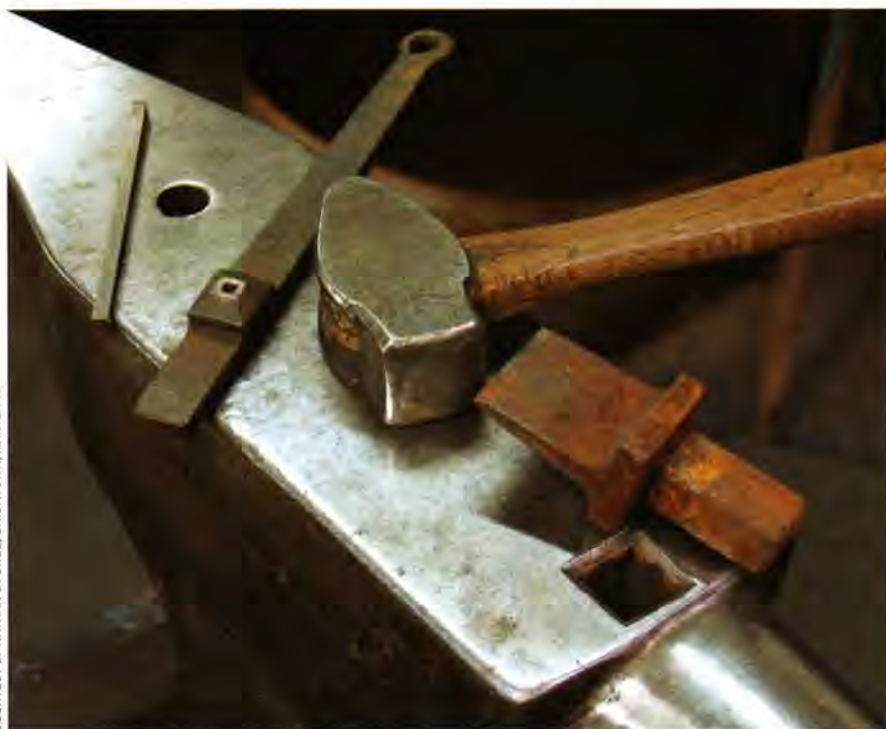
Nick Vincent of Nathan's Forge uses tools typical of an 18th-Century nailsmith. Resting on top of the heavy anvil, from top, are a piece of nail rod, a nail header, a blacksmith's hammer, and a hardy.
